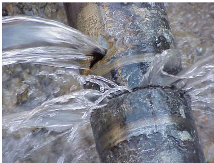
Aging infrastructure like this leaky pipeline contributes to system losses and unrecovered cost for municipalities.
